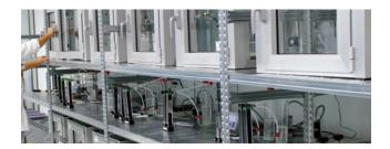
room in Europe, developed alongside the Engineering Department of the University of Modena and Reggio Emilia (EELab, Energy Efficiency Laboratory), which is capable of determining the actual energy performance levels of a properly insulated wall.
