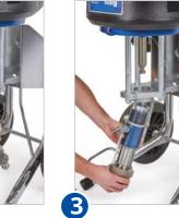
Rotate the pump to remove it
