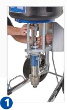
Remove joint paint inlet and
